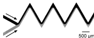
FIGURE 1. Optical micrograph of two-phase laminar flow: two aqueous phases, each colored with a different dye (black ink and Congo red), brought together with a “Y” junction in an elastomeric microfluidic system.
